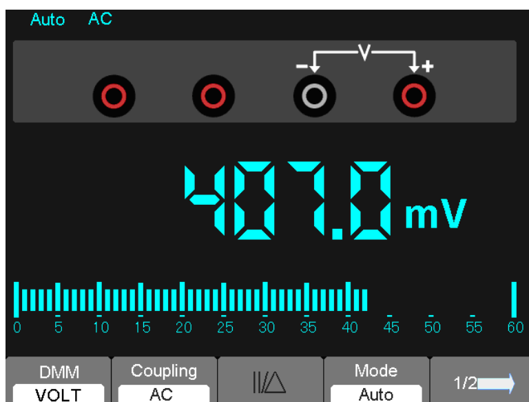
Figure 7-7 AC voltage Measurement
